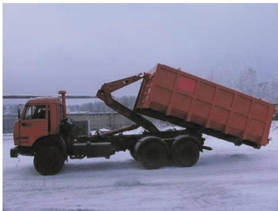
3.13-rasm. Multilift tizim bilan jhozlangan chiqindi mashinasi
