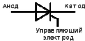
1-rasm. Tiristor (trinistor)ning belgilanishi
