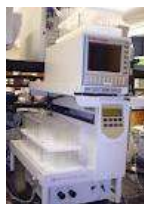
Zamonaviy suv oqimi xromatografi (flush purification system)
