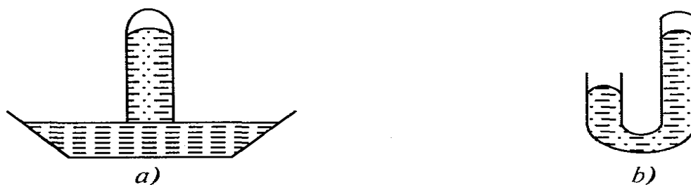
1. 1-rasm. Simobli barometr: a) idishli, b) sifonli.
