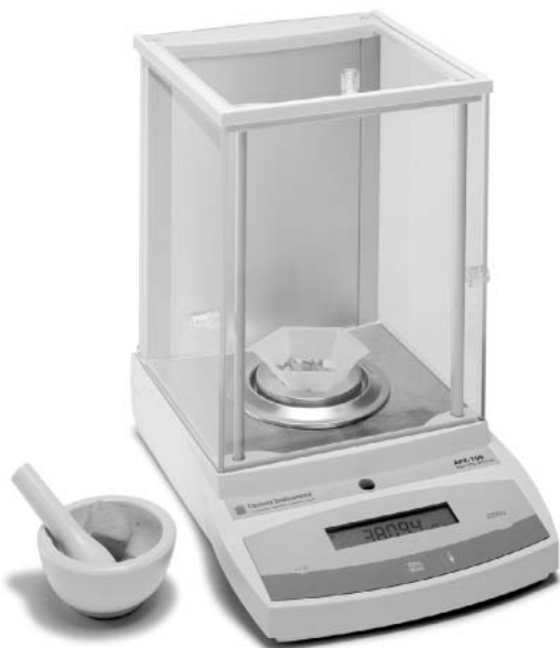
Fig. 2.1. Electronic analytical balance. (Courtesy of Denver Instrument Co. Denver Instrument Company owns all images.)
