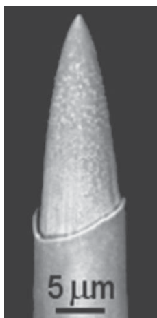
Fig. 15.7. CarboStar 1, voltammetric carbon fiber ultramicroelectrode. Courtesy of Kation Scientific USA ( www.Kationscientific.com ).
