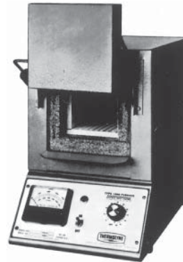
Fig. 2.13. Muffle furnace. (Courtesy of Arthur H. Thomas Company.)
