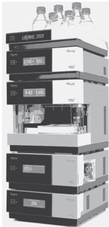
Fig. 21.2. A modular (U)HPLC system. From top: solvent tray and degasser, gradient pump (binary or quaternary), thermostated autosampler, thermostated column compartment with automated switching valve(s), UV–Vis absorbance detector. (Courtesy of Thermo Fisher Scientific Inc.)
