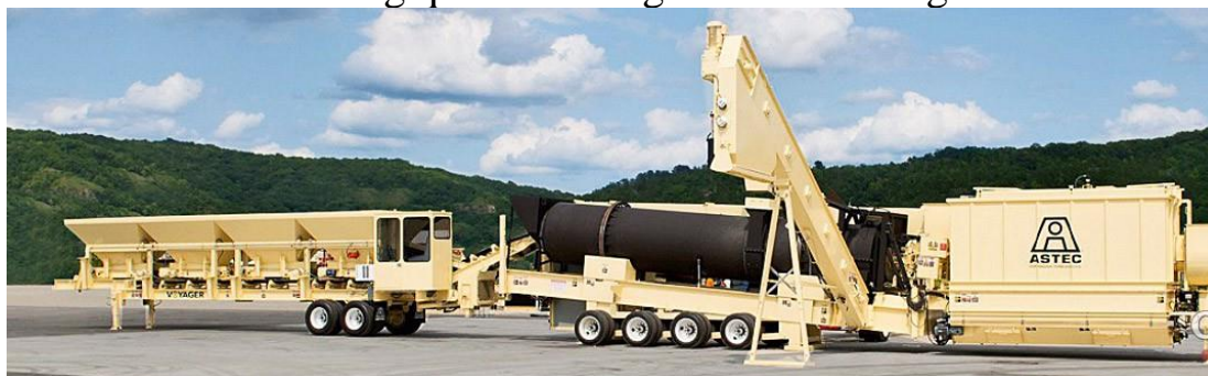
3.9-rasm. Voyager Astec asfaltbeton qarishmalarini tayyorlash zavodi
