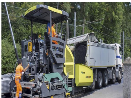
1.24-rasm. Ammann kompaniyasining AFT 900-3 markali asfaltyotqizgichi
