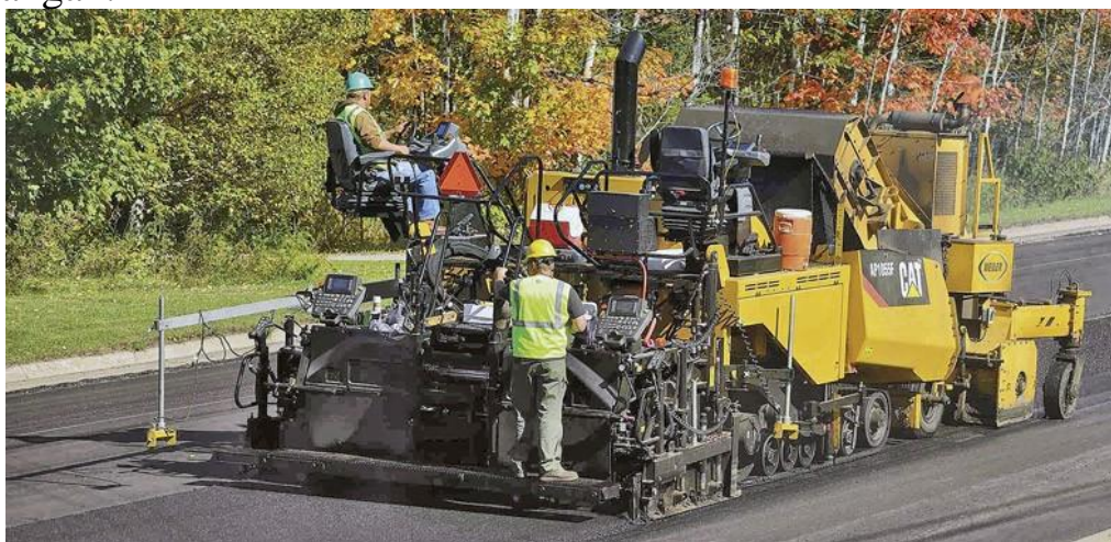
1.29-rasm. Caterpillar kompaniyasining AP 655D markali asfaltyotqizgichi
