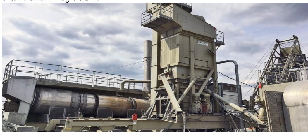
3.6-rasm. ABZ ROADBATCHE 160 na avtomobilnom shassi ot ERMONT
