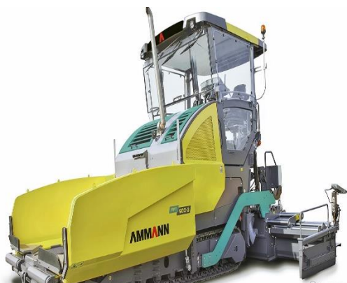
1.24-rasm. Ammann kompaniyasining AFT 900-3 markali asfaltyotqizgichi
