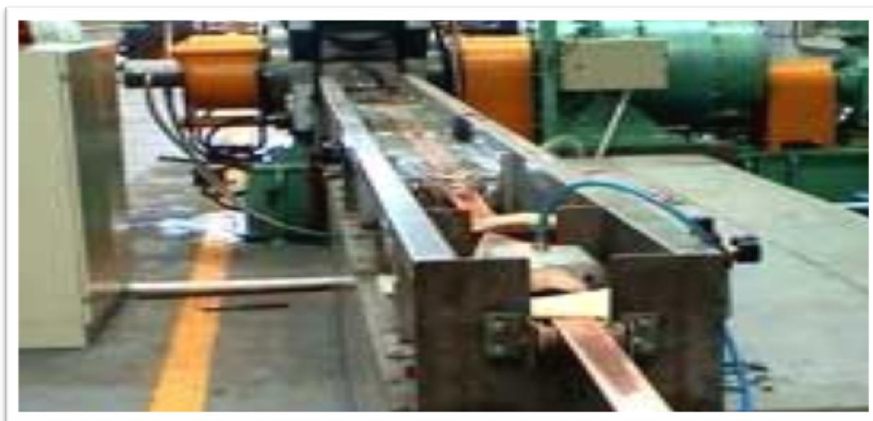
6.8-rasm. Ikkilamchi mis tarkibli temir-tersak va chiqindilarga ishlov berish.
