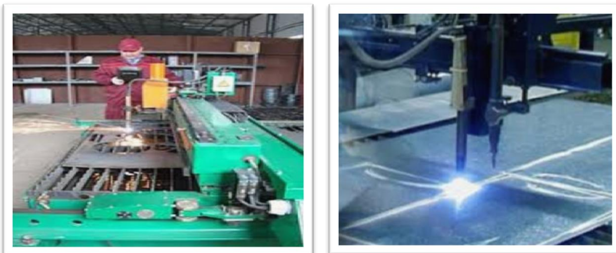
4.7-rasm. Plazmali-yoyli aligatorlarda qirqish
