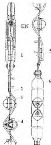
14.3-rasm. PKS105 lentali kumulyativ perforator:
