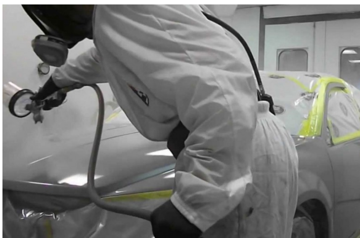
17.11-rasm. Avtomobil kuzoviga nanokukunli (zarrachali) himoya qatlami berilishi
