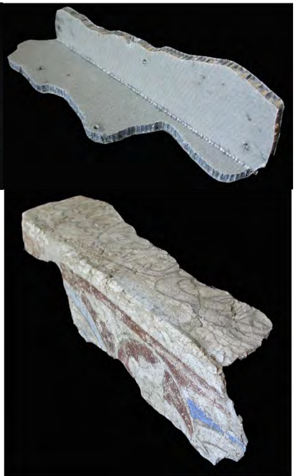
Fig.15. Preparation of the aluminum sheet for an architectural fragment
