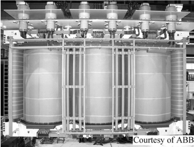
Figure 4-6 Transformer core and coils. Courtesy of ABB.
