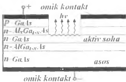
9.15-rasm. Vertikal rezonatorli nanoelektron lazer tuzilishi.
