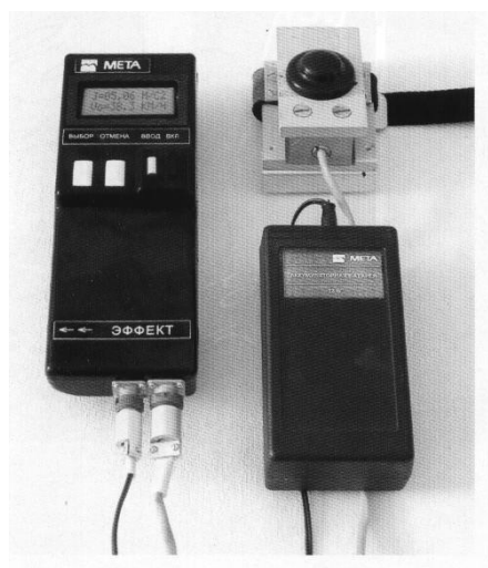
11.2-rasm. Tormoz tizimining samaradorligini aniqlovchi Effekt- 02 jihozi
