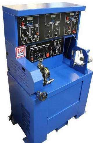
8.1-rasm. E250M-02 modelidagi generator va starterni tekshiruv-nazorat stend
