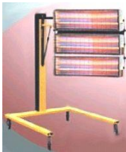
5.4-rasm. Kuzovni qisman IQ- quritish ustuni
