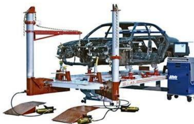
4.3-rasm. Kuzovlarni to'g'rilash jihozi
