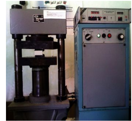
7-rasm. Gidravlik press: 5-ustki tayanch plita, 6-namunani mahkamlaydigan burama moslama, 7-manometr, 8-nasos. 1-stanina, 2-porshen, 3-pastki tayanch plita, 4-sinalayotgan namuna,
