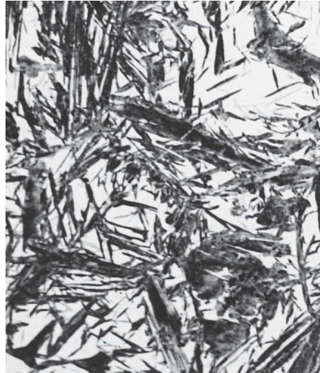
Figure 10.21 Photomicrograph showing the martensitic microstructure. The needle-shape grains are the martensite phase, and the white regions are austenite that failed to transform during the rapid quench. 1220 \times . (Photomicrograph courtesy of United States Steel Corporation.)
