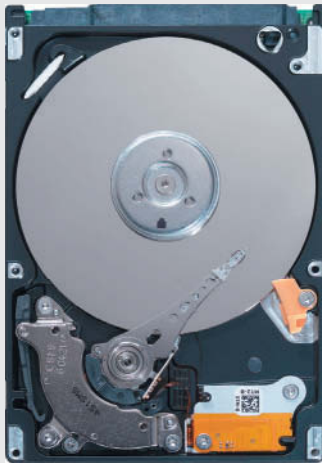
(c) The inside of a hard disk drive. The circular disk will typically spin at a rotational velocity of 5400 or 7200 revolutions per minute.
