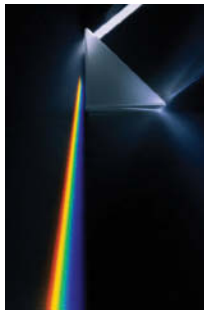
The dispersion of white light as it passes through a prism. (© PhotoDisc/Getty Images.)
