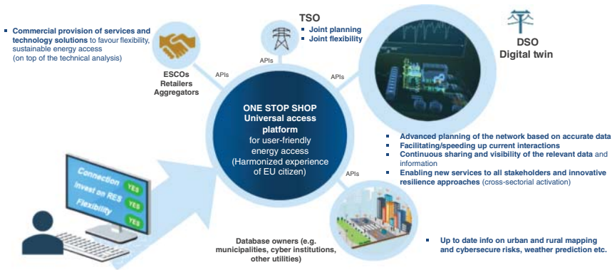
Figure 6.19 The OSS “one-stop shop” network supporting the universal access of the users to the local and EU market offers of energy services companies, retailers, aggregators, and others. Backoffice complex integration between TSOs, DSOs, ESCOs, and market actors leads to simple front-office access for end users.
