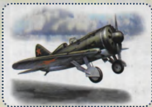
I-16 qiruvchi samolyoti – monoplan
