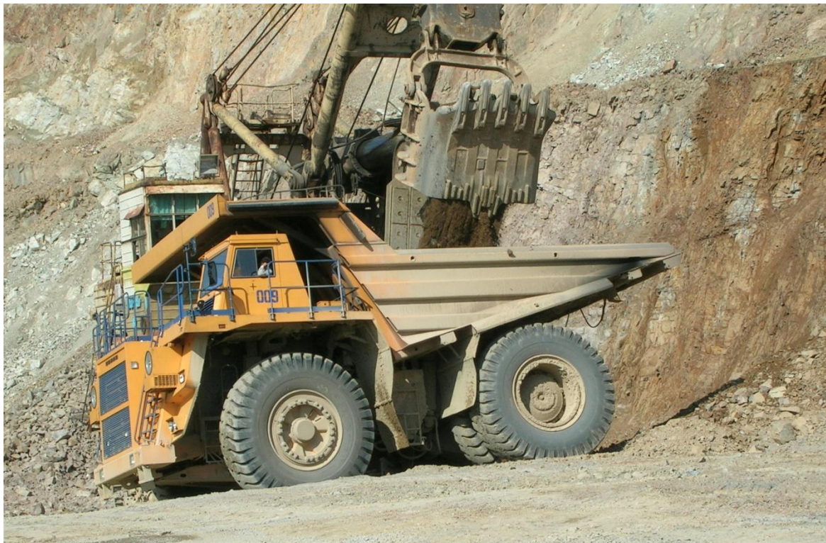
11.1. Rasm. Karer avtomobil transportining ish jarayoni.
