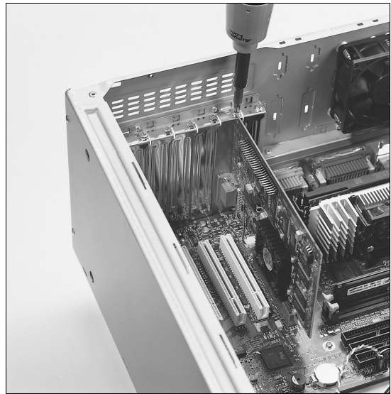
Figure 22.28 Installing the screw to retain the card. Motherboard courtesy of Intel Corporation.
