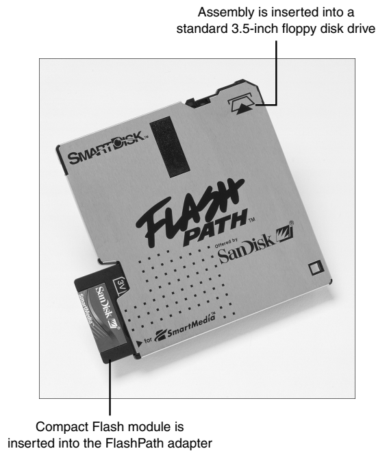
Figure 12.6 A CompactFlash module is inserted into the FlashPath adapter; the assembly is then inserted into a standard 3 1/2" floppy drive. Photo courtesy of SanDisk.
