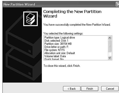
Figure 14.10 The New Partition Wizard prepares to format a logical drive on Disk 1 with the options shown.
