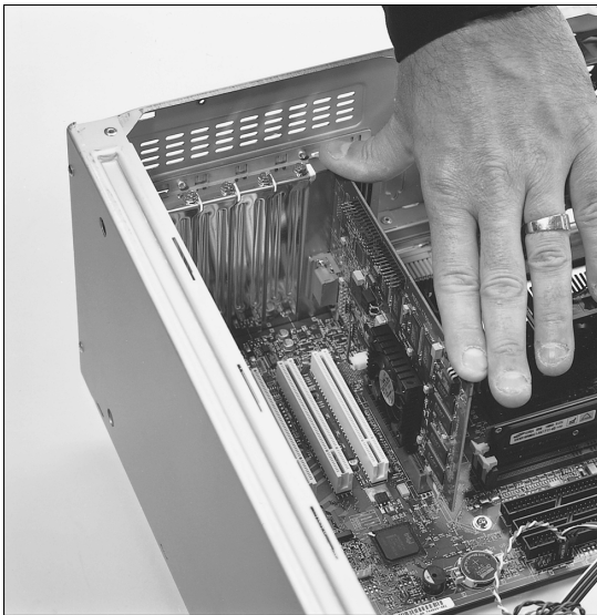
Figure 22.27 This photo shows a video adapter being inserted into the slot. Motherboard courtesy of Intel Corporation.
