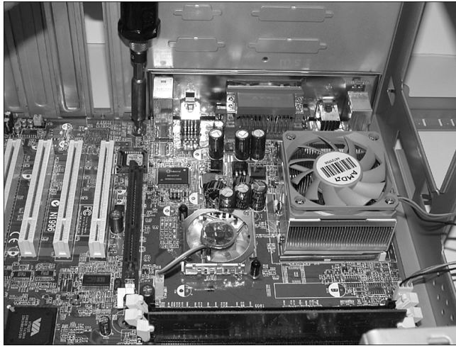
Figure 22.18 Installing the screws that hold the motherboard to the chassis.
