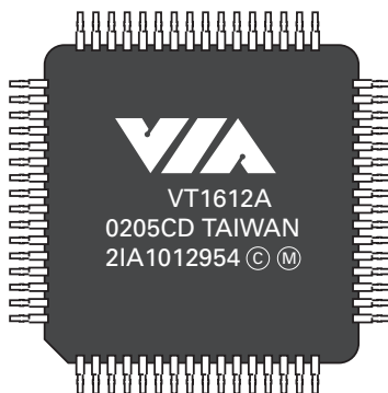
Figure 16.8 The VIA VT1612A is a typical AC'97 2.2-compliant codec chip (foreground), seen here providing integrated audio for the VIA EPIA-V Mini-ITX motherboard (background). Photos courtesy of VIA Technologies, Inc.
