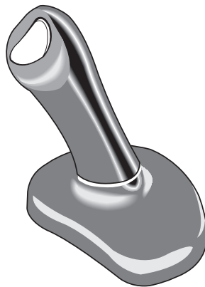
Figure 18.14 The 3M Ergonomic Mouse combines an ergonomic shape with a standard mouse-movement mechanism.
