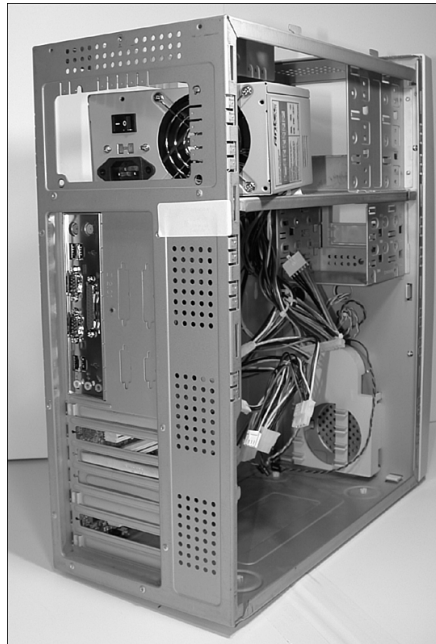
Figure 22.19 Installing the power supply into the chassis.
