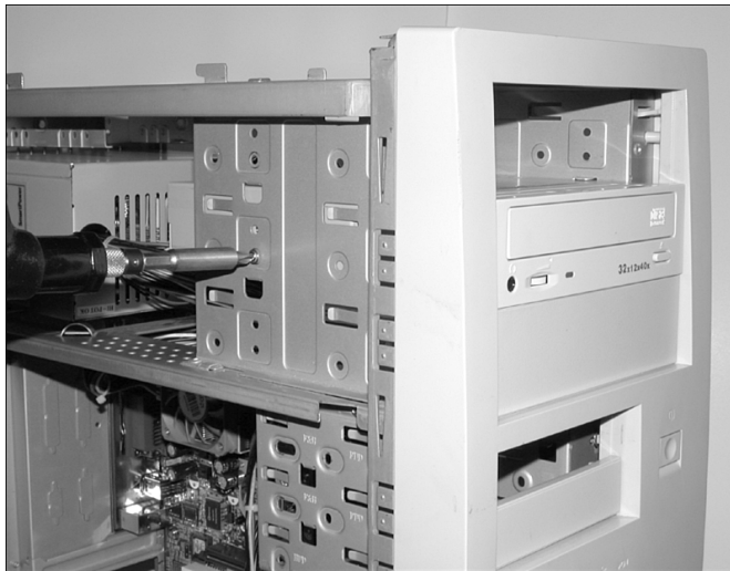
Figure 22.24 Secure the drive to the chassis using four screws.
