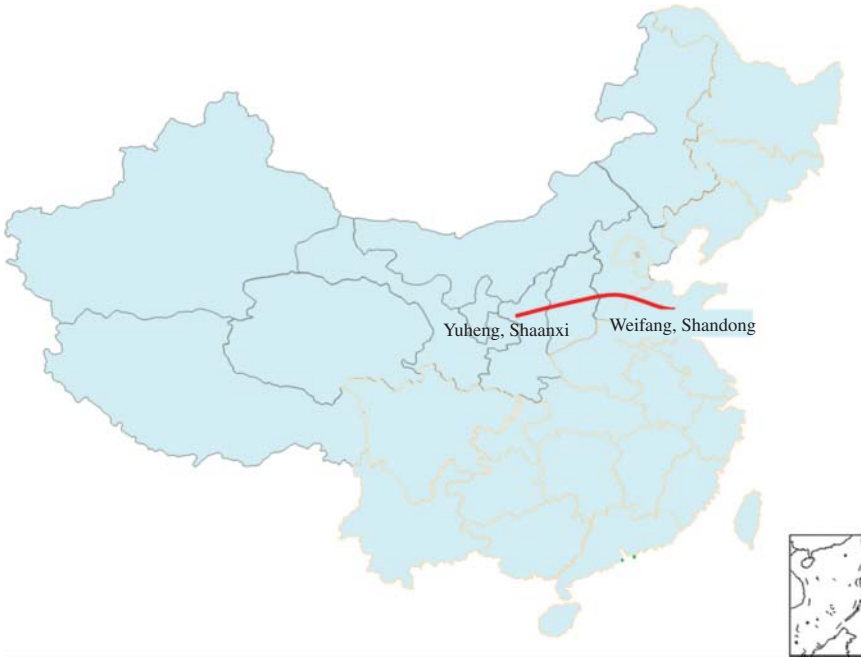
Figure 2.29 Yuheng-Weifang 1000 kV UHV AC project (under construction) (transmission capacity: 10 GW, distance: 1049 km). Picture source: SGCC.
