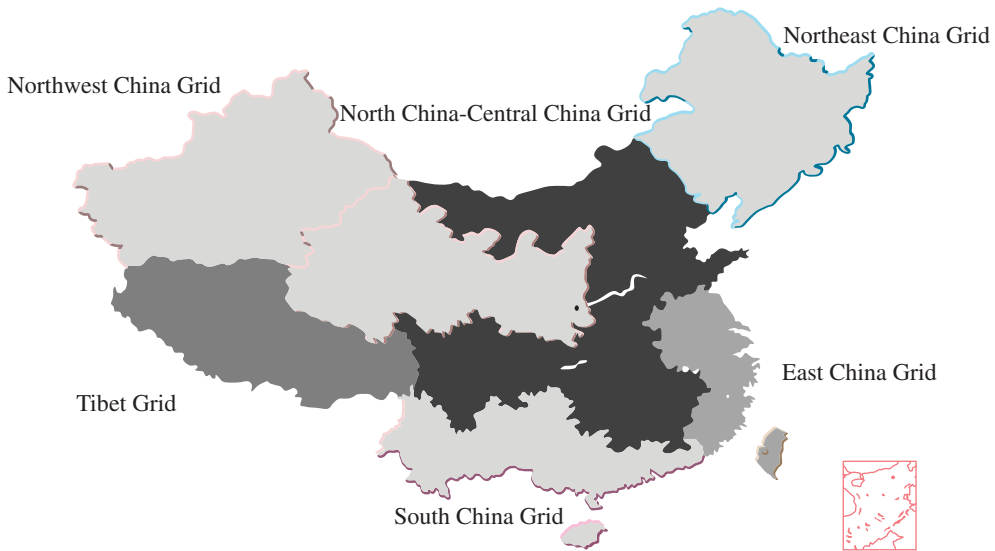
Figure 1.31 Schematic diagram of the interconnection of China's power grids in 2015. Picture source: SGCC.
