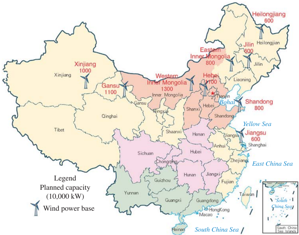
Figure 2.38 China's wind power bases with a planned capacity of above 10 GW. Data source: China Electricity Council.
