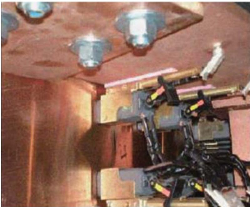
Figure A.8 Connection diagram of the brush and collector ring of a VFT [5].
