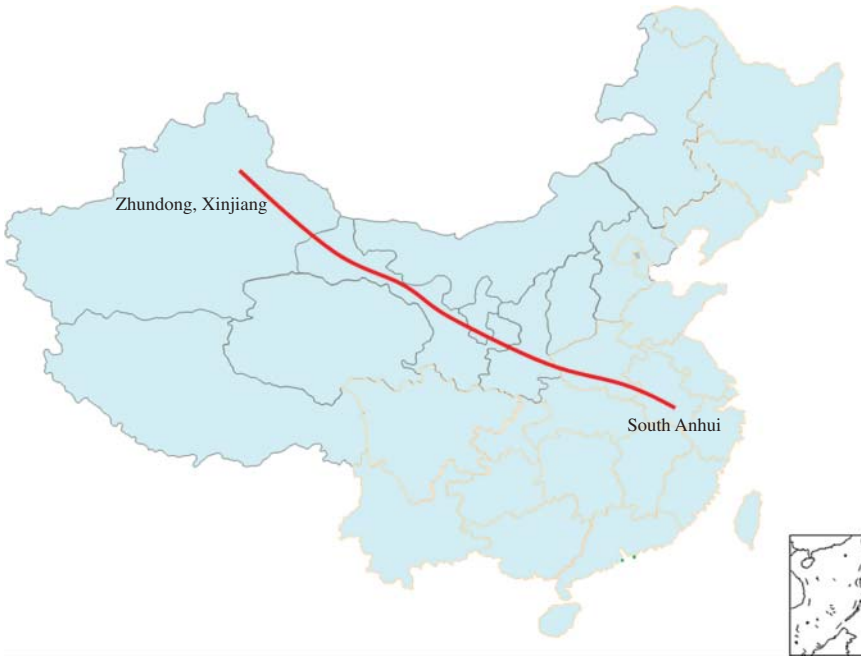
Figure 2.30 Zhundong-South Anhui \pm 800 kV UHV DC project (under construction) (transmission capacity: 12 GW, distance: 3324 km). Picture source: SGCC.
