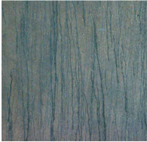
Fig. 21.7 Arc tracks on a lower W-coated (1 μm) tile of the divertor baffle of ASDEX Upgrade. Figure taken from [40]. Used with permission
