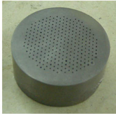
Fig. 22.32 Photograph of the Ta shower-head cap-shaped anode with 0.6 mm diameters of 250 holes
