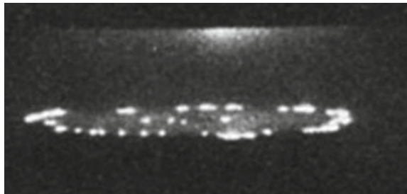
Fig. 13.15 Expanding ring of cathodic spots: current, 5.3 kA; ring diameter, 50 mm [47]
