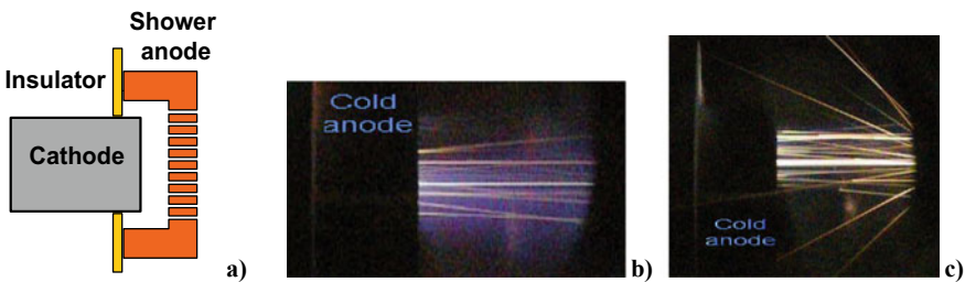
Fig. 9.20 Schematic cathode-anode presentation (a), MP’s ejection from the shower anode at initial cold stage (b), MP’s reflection from the shutter placed between the anode front surface and a substrate (c)
