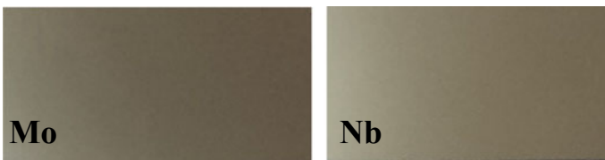
Fig. 22.48 Photograph of Mo and Nb films obtained using configuration a with a 200 A arc, L = 110 mm
