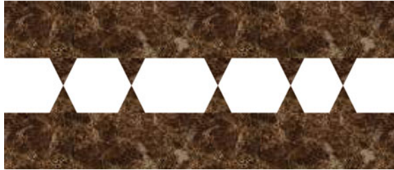
Fig. 6.1 Schematic presentation of the contact of not ideally smooth surfaces
