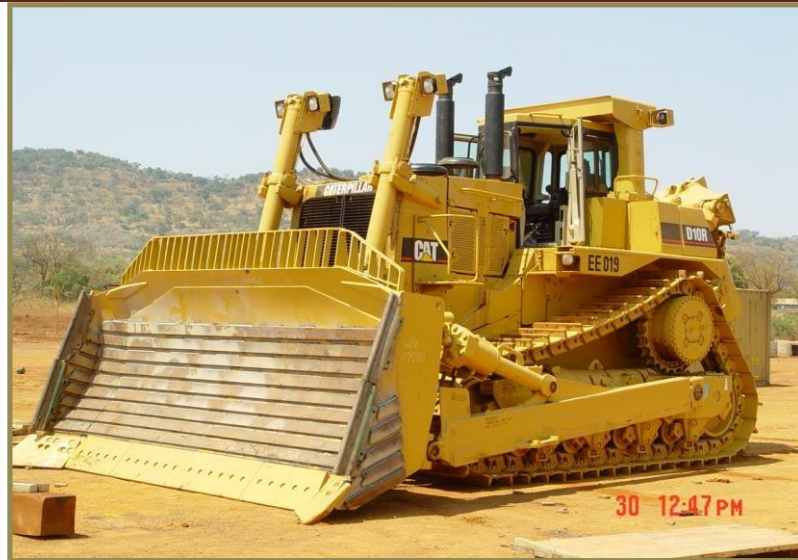
5.5 – rasm. Karyerda buldozerning ish jarayoni.
