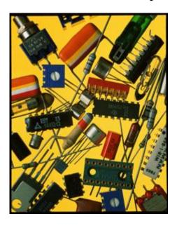
Discrete (meaning separate) electronic components can be selected individually and put together to make a circuit. Examples of discrete components include resistors, capacitors, diodes and transistors.
