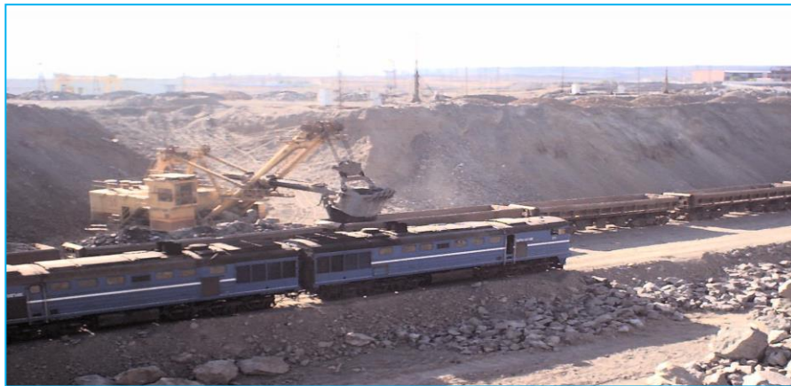
5.4 – rasm. Karyerda temir yo‘l transportining ish jarayoni.
