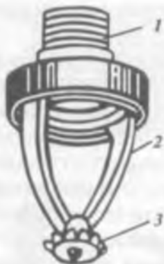
79-rasm. Suv bilan o'chiruvchi drencher kallagi:
