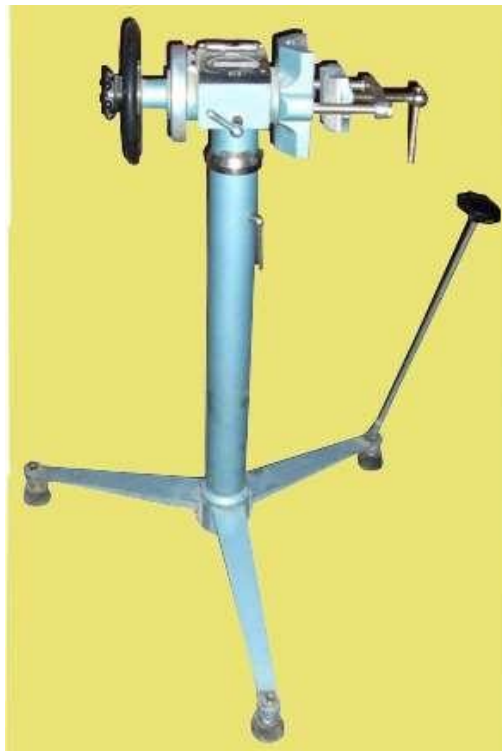
15.7-rasm. Inklinometrni darajalash stoli (USI-2)
