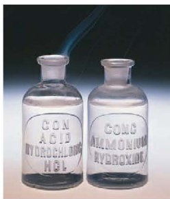
▲ Figure 16.3 A gas-phase acid–base reaction. The \text{HCl}(g) escaping from concentrated hydrochloric acid and the \text{NH}_3(g) escaping from aqueous ammonia (here labeled ammonium hydroxide) combine to form a white fog of \text{NH}_4\text{Cl}(s) .
