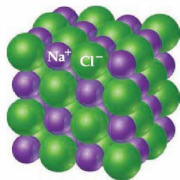
▲ Figure 8.3 The crystal structure of sodium chloride. In this three-dimensional array of ions, each \text{Na}^+ ion is surrounded by six \text{Cl}^- ions, and each \text{Cl}^- ion is surrounded by six \text{Na}^+ ions.
