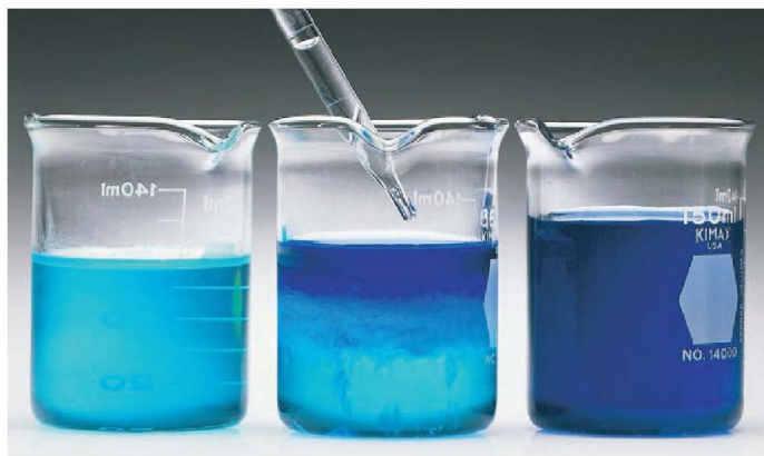
▲ Figure 24.22 Effect of ligands on color. An aqueous solution of \text{CuSO}_4 is pale blue because of [\text{Cu}(\text{H}_2\text{O})_4]^{2+} (left). When \text{NH}_3(aq) is added (middle and right), the deep blue [\text{Cu}(\text{NH}_3)_4]^{2+} ion forms.
