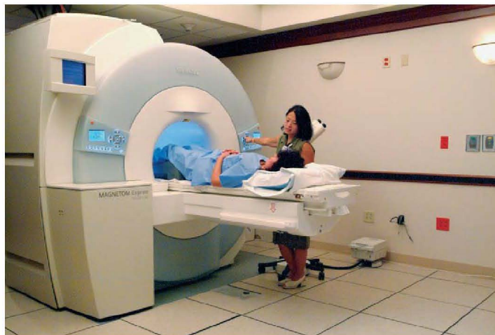
▶ Figure 12.19 A magnetic resonance imaging (MRI) machine used in medical diagnosis. The magnetic field needed for the procedure is generated by current flowing in superconducting wires, which must be kept below their superconducting transition temperature, T_c , of 18 K. This low temperature requires liquid helium as a coolant.
