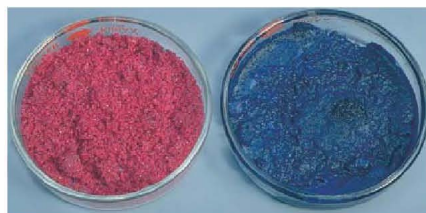
▲ Figure 13.8 Hydrates and anhydrous salts. Hydrated cobalt(II) chloride, \text{CoCl}_2 \cdot 6 \text{H}_2\text{O} (left), and anhydrous \text{CoCl}_2 (right).
