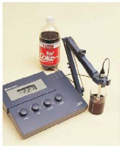
▲ Figure 16.6 A digital pH meter. The device is a millivoltmeter, and the electrodes immersed in the solution being tested produce a voltage that depends on the pH of the solution.
