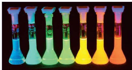
▲ Figure 12.44 Semiconductor nanoparticles of CdS of different sizes. When illuminated with ultraviolet light, these solutions of semiconductor nanoparticles emit light that corresponds to their respective band gap energies.
