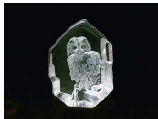
▲ Figure 22.13 Etched, or frosted, glass. Designs such as this are produced by first coating the glass with wax and then removing the wax only in the areas to be etched. When treated with hydrofluoric acid, the exposed areas of the glass are attacked, producing the etching effect.
