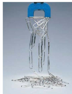
▲ Figure 23.24 Permanent magnets. Permanent magnets are made from ferromagnetic and ferrimagnetic materials.
