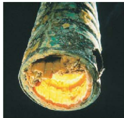
◀ Figure 18.21 Scale formation. A section of water pipe that has been coated on the inside with \text{CaCO}_3 and other insoluble salts deposited from hard water.
