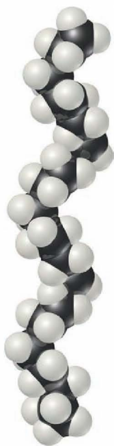
▲ Figure 12.24 A segment of a polyethylene chain. The segment shown here consists of 28 carbon atoms. In commercial polyethylenes the chain lengths range from about 10^3 to 10^5 \text{CH}_2 units. As this illustration implies, the chains are flexible and can coil and twist in random fashion, which makes it difficult to see all 28 carbons in this illustration.
