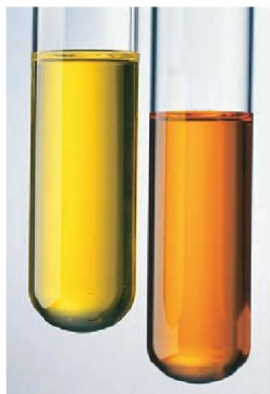
▲ Figure 23.26 Chromate and dichromate solutions. Solutions of sodium chromate, \text{Na}_2\text{CrO}_4 (left), and potassium dichromate, \text{K}_2\text{Cr}_2\text{O}_7 (right), illustrate the difference in color of the chromate and dichromate ions.
