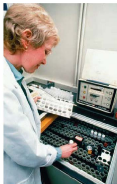
▲ Figure 21.12 A scintillation counter. Such counters are used to quantitatively measure the level of radiation.
