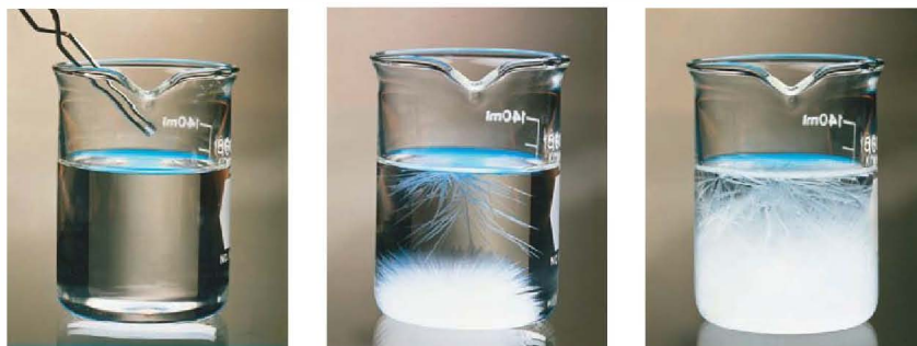
(a) A seed crystal of \text{NaCH}_3\text{COO} being added to the supersaturated solution. (b) Excess \text{NaCH}_3\text{COO} crystallizes from the solution. (c) The solution arrives at saturation.
