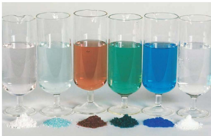
▲ Figure 23.21 Salts of transition-metal ions and their solutions. From left to right: \text{Mn}^{2+} , \text{Fe}^{2+} , \text{Co}^{2+} , \text{Ni}^{2+} , \text{Cu}^{2+} , and \text{Zn}^{2+} .
