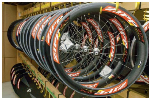
▲ Figure 22.40 Carbon composites. Carbon composites are used extensively in aerospace and automotive applications and in sporting goods. These high-performance (and high-priced!) bike wheels have a carbon-fiber-composite frame, which makes them very lightweight and helps them absorb road shocks.
