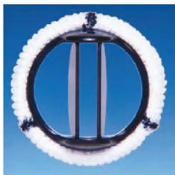
▲ Figure 12.33 A disc heart valve. Known as the St. Jude valve, this device was named for the medical center at which it was developed. The surfaces of the valve are coated with pyrolytic carbon. The valve is secured to the surrounding tissue via a Dacron® sewing ring.
