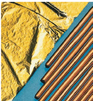
▲ Figure 23.12 Malleability and ductility. Gold leaf (left) demonstrates the characteristic malleability of metals, and copper wire (right) demonstrates their ductility.
