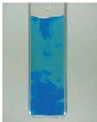
▲ Figure 23.29 Precipitation of Cu(OH) 2 . Addition of NaOH solution to an aqueous solution of Cu 2+ causes Cu(OH) 2 to precipitate.
