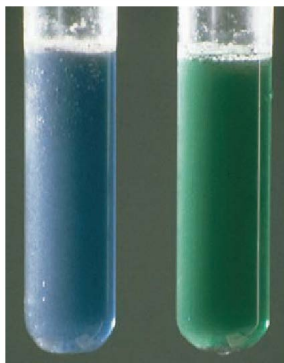
▲ Figure 23.25 Two forms of the Cr(III) ion . The tube on the left contains the violet hydrated chromium(III) ion, \text{Cr}(\text{H}_2\text{O})_6^{3+} . The tube on the right contains the green [(\text{H}_2\text{O})_4\text{Cr}(\text{OH})_2\text{Cr}(\text{H}_2\text{O})_4]^{4+} ion.
