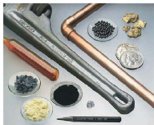
▲ Figure 2.17 Some familiar examples of metals and nonmetals. The nonmetals (from bottom left) are sulfur (yellow powder), iodine (dark, shiny crystals), bromine (reddish brown liquid and vapor in glass vial), and three samples of carbon (black charcoal powder, diamond, and graphite in the pencil lead). The metals are in the form of an aluminum wrench, copper pipe, lead shot, silver coins, and gold nuggets.
