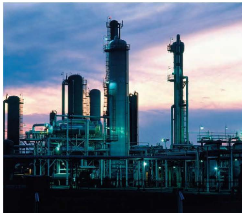
▲ Figure 13.21 Separating volatile components. In an industrial distillation tower, such as the ones shown here, the components of a volatile organic mixture are separated according to boiling-point range.
