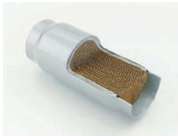
▲ Figure 14.22 Cross section of a catalytic converter. Automobiles are equipped with catalytic converters, which are part of their exhaust systems. The exhaust gases contain CO, NO, \text{NO}_2 , and unburned hydrocarbons that pass over surfaces impregnated with catalysts. The catalysts promote the conversion of the exhaust gases into \text{CO}_2 , \text{H}_2\text{O} , and \text{N}_2 .
