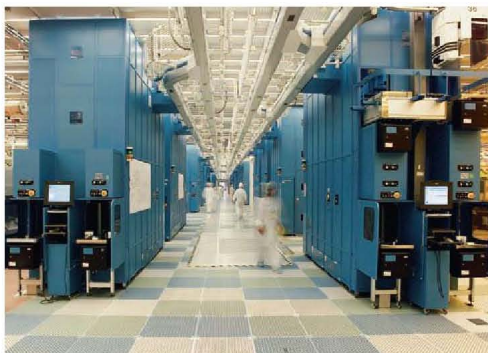
▲ Figure 12.9 Making silicon chips. IBM's clean room for the fabrication of 300 mm silicon wafers, in East Fishkill, New York. Tam Way/Courtesy of International Business Machines Corporation. Unauthorized use not permitted.
