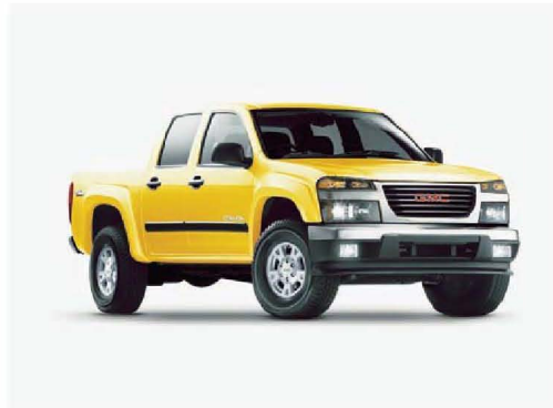
▲ Figure 12.31 A mostly plastic truck. This truck has door handles and bumper supports made of polycarbonate/polybutylene plastic. Coloring pigments are incorporated into the manufacture of the plastic, eliminating the need for painting.
