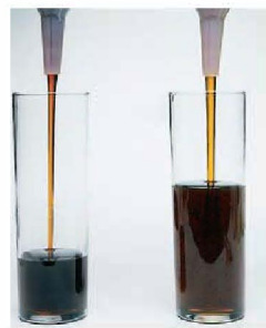
▲ Figure 11.13 Comparing viscosities. The Society of Automotive Engineers (SAE) has established numbers to indicate the viscosity of motor oils. The higher the number, the greater the viscosity is at any given temperature. The SAE 40 motor oil on the left is more viscous and flows more slowly than the less viscous SAE 10 oil on the right.
