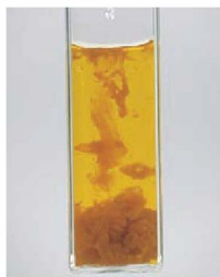
▲ Figure 23.27 Precipitation of Fe(OH) 3 . Addition of NaOH solution to an aqueous solution of Fe 3+ causes Fe(OH) 3 to precipitate.
