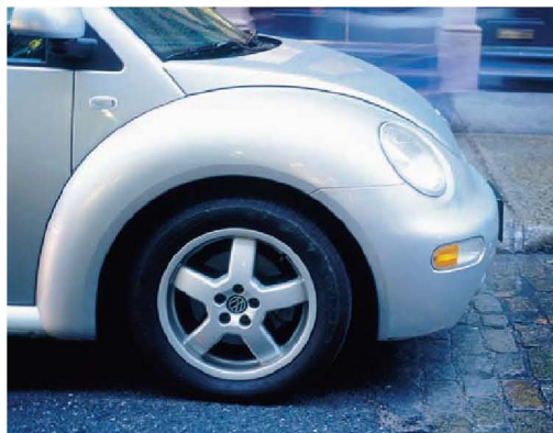
▲ Figure 12.30 Plastic fenders. The fenders of this Volkswagen Beetle are made of General Electric Noryl GTX, a composite of nylon and polyphenylene ether.
