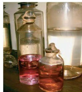
▶ Figure 12.47 The solutions of colloidal gold nanoparticles made by Michael Faraday in the 1850s. These are on display in the Faraday Museum, London.
