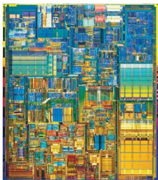
▲ Figure 12.8 Photograph of a Pentium 4 processor computer chip. On this scale, mostly what you can see is the connections between transistors.
