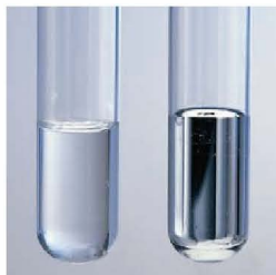
▲ Figure 11.16 Two meniscus shapes. The water meniscus in a glass tube compared with the mercury meniscus in a similar tube. Water wets the glass, and the bottom of the meniscus is below the level of the water–glass contact line, giving a U-shape to the water surface. Mercury does not wet glass and the meniscus is above the mercury–glass contact line, giving an inverted U-shape to the mercury surface.
