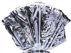
▲ Figure 7.22 Elemental silicon. Silicon is an example of a metalloid. Although it looks metallic, silicon is brittle and is a poor thermal and electrical conductor as compared to metals. Large crystals of silicon are sliced into thin wafers for use in integrated circuits.
