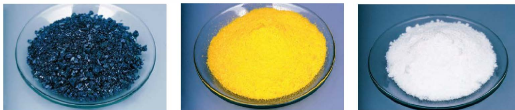
▲ Figure 24.36 Effect of charge-transfer transitions. The compounds \text{KMnO}_4 , \text{K}_2\text{CrO}_4 , and \text{KClO}_4 are shown from left to right. The \text{KMnO}_4 and \text{K}_2\text{CrO}_4 are intensely colored because of ligand-to-metal charge transfer (LMCT) transitions in the \text{MnO}_4^- and \text{CrO}_4^{2-} anions. There are no valence d orbitals on Cl, so the charge-transfer transition for \text{ClO}_4^- requires ultraviolet light and \text{KClO}_4 is white.
