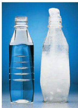
▲ Figure 11.11 Expansion of water upon freezing. Water is one of the few substances that expand upon freezing. The expansion is due to the open structure of ice relative to that of liquid water.
