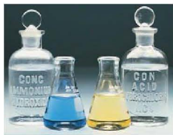
▲ Figure 4.7 The acid–base indicator bromthymol blue. The indicator is blue in basic solution and yellow in acidic solution. The left flask shows the indicator in the presence of a base, aqueous ammonia (labeled as ammonium hydroxide). The right flask shows the indicator in the presence of hydrochloric acid, \text{HCl} .
