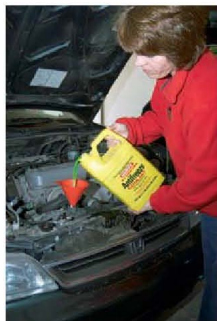
Antifreeze being added to an automobile radiator. Antifreeze consists of an aqueous solution of ethylene glycol, \text{CH}_2(\text{OH})\text{CH}_2(\text{OH}) .
