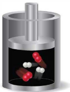
▲ Figure 5.3 A closed system and its surroundings. Hydrogen and oxygen gases are confined in a cylinder with a movable piston. If we are interested only in the properties of these gases, the gases are the system and the cylinder and piston are part of the surroundings. Because the system can exchange energy (in the form of heat and work) but not matter with its surroundings, it is a closed system.
