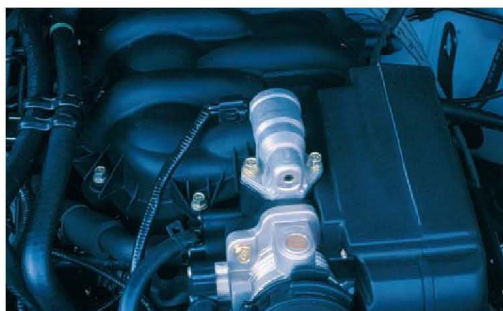
▲ Figure 12.29 Plastic engines. The intake manifold of some Ford V-8 engines is formed from nylon.
