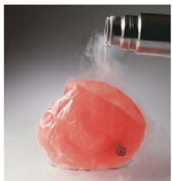
▲ Figure 10.8 An illustration of the effect of temperature on volume. As liquid nitrogen ( -196\text{ }^{\circ}\text{C} ) is poured over a balloon, the gas in the balloon is cooled and its volume decreases.
