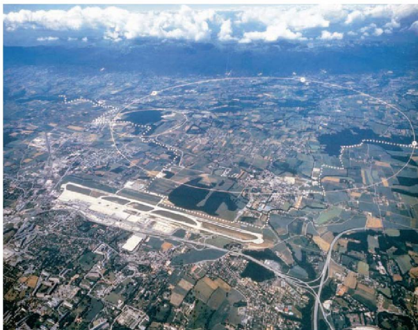
▲ Figure 21.7 CERN (Conseil Européen pour la Recherche Nucléaire), Geneva, Switzerland. Particles are accelerated to very high energies by circulating them through magnets in the ring, which has a circumference of 27 km.
