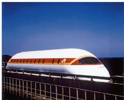
▲ Figure 12.18 Superconduction in action. High speed superconductive magnetic levitation (maglev) train. Shown is the ML002 experimental train being tested in Japan.
