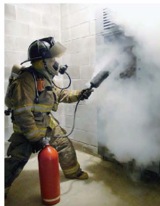
▲ Figure 10.14 A \text{CO}_2 fire extinguisher. The \text{CO}_2 gas from a fire extinguisher is denser than air. The \text{CO}_2 cools significantly as it emerges from the tank. Water vapor in the air is condensed by the cool \text{CO}_2 gas and forms a white fog accompanying the colorless \text{CO}_2 .
