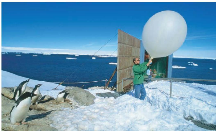
◀ Figure 10.5 An application of the pressure-volume relationship. The volume of gas in this weather balloon will increase as it ascends into the high atmosphere, where the atmospheric pressure is lower than on Earth's surface.
