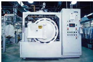
▲ Figure 18.22 Green chemistry for your clothes. This dry-cleaning apparatus employs liquid CO 2 as the solvent.
