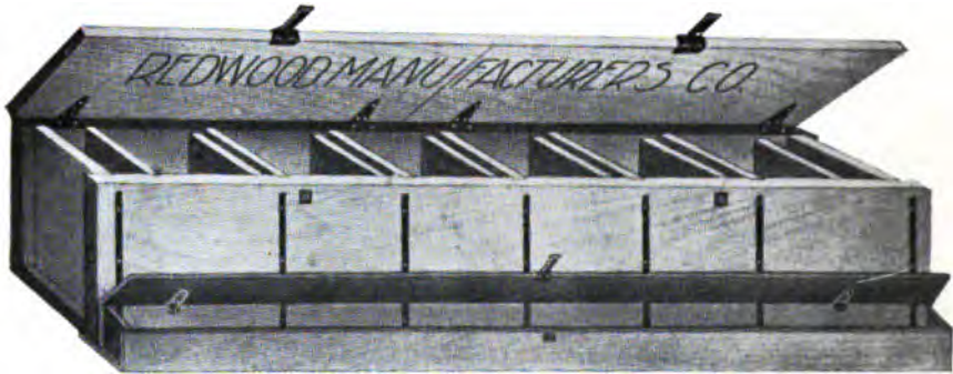
FIG. 75. PERSPECTIVE VIEW OF ZINC BOXES.
