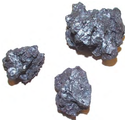
Figure 1.1.10 Typical sinter for blast furnace process (size: \leq 25 mm) [22].
