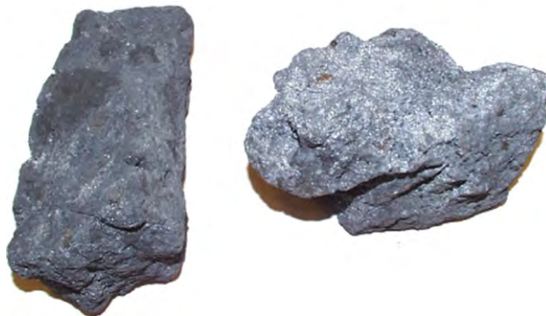
Figure 1.1.13 Coke particles for blast furnace process [22].
