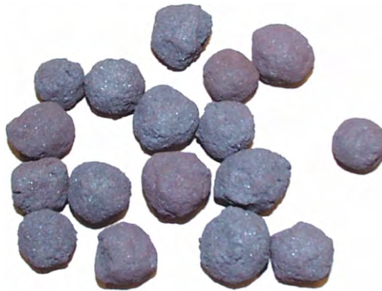
Figure 1.1.12 Iron ore pellets (size: 9–13 mm) [22].
