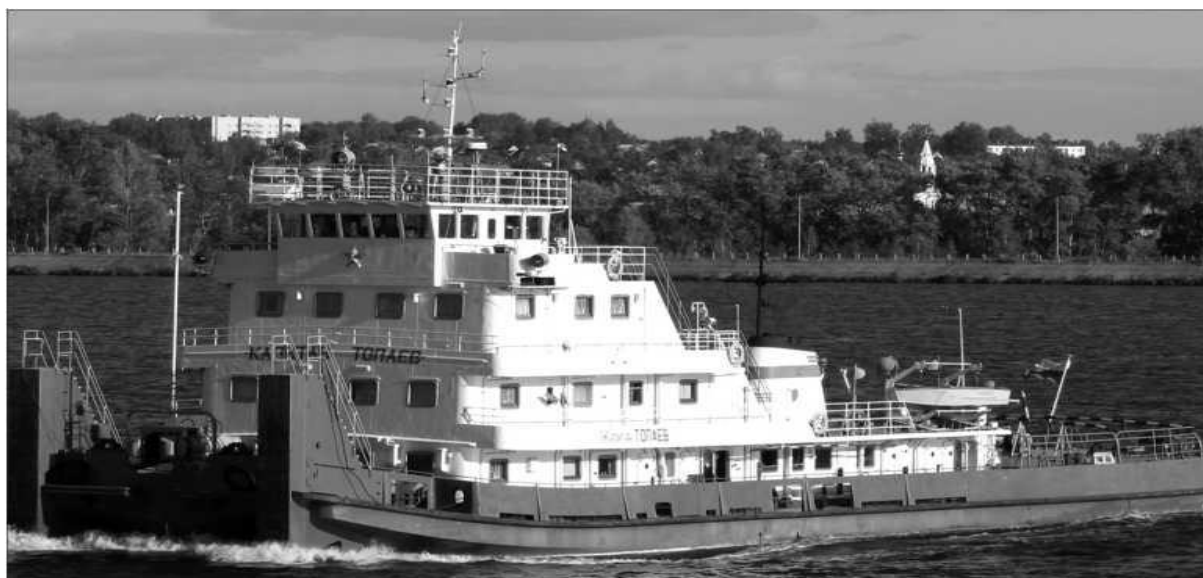
3.3-rasm. Tolkach-buksir 428 quvvati 2000 ot kuchi.
