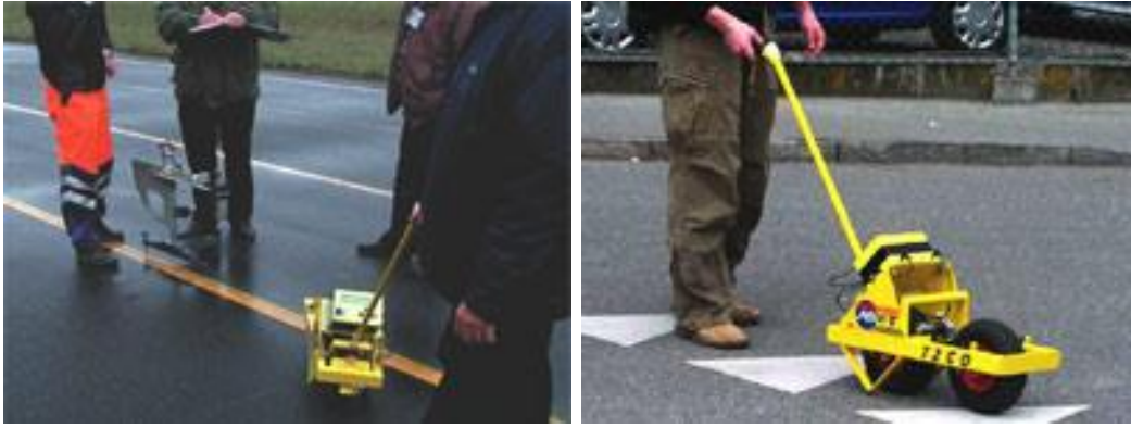
2.12-rasm. T2GO portativ qurilmasining Cooper Pendulum Skid Resistance tester qurilmasi bilan solishtirish jarayoni
