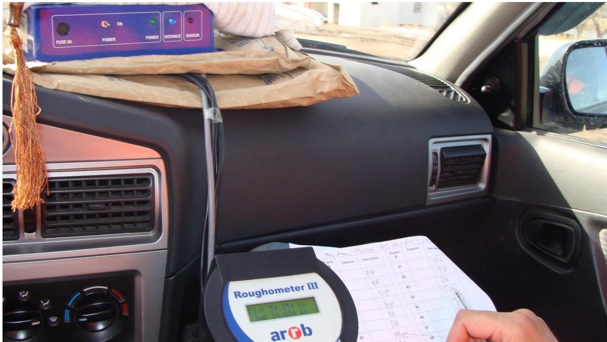
Roughometer III qurilmasi yordamida ravonlikni o'lchash jarayoni
