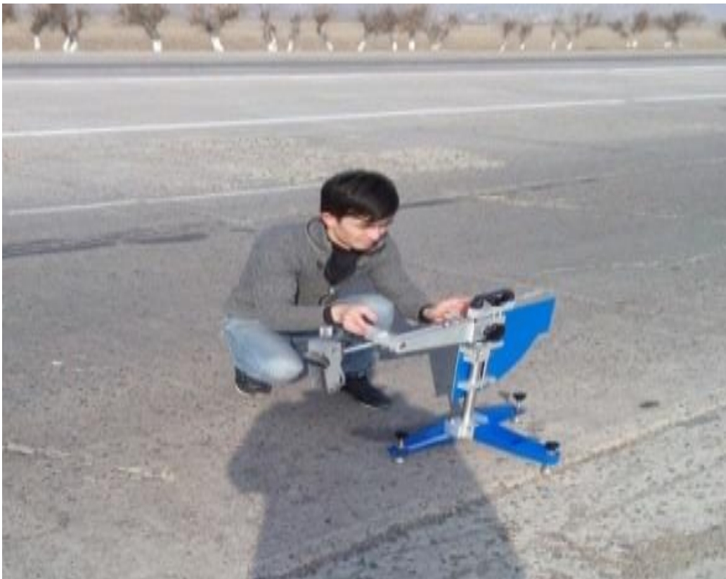
Cooper Pendulum Skid Tester qurilmasi yordamida asfaltbeton qoplamasining tishlashish sifatini o'lchash jarayoni
