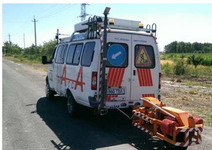
2.8-rasm. PKRS-2U turidagi dinomometrik tirkamasining maxsus laboratoriya avtomobiliga ulangan ishchi holatdagi ko'rinishi
