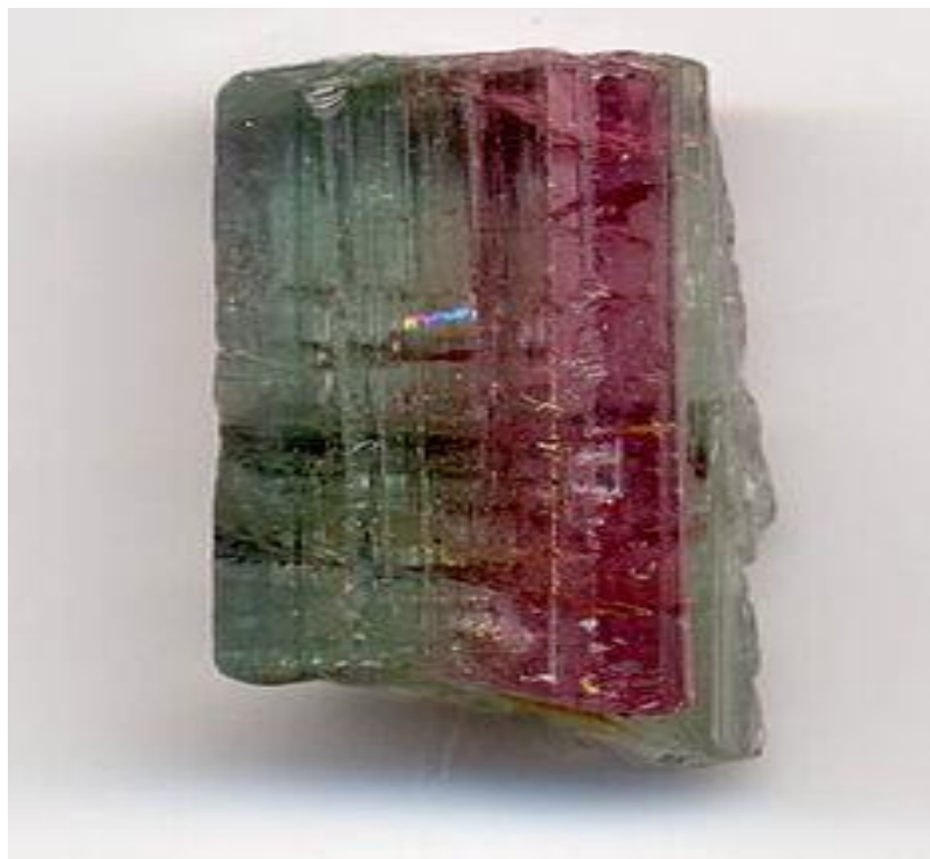
25 - rasm. Turmalin - \text{Na}(\text{Li},\text{Al})_3\text{Al}_6[(\text{OH})_4(\text{BO}_3)_3\text{Si}_6\text{O}_{18}]
