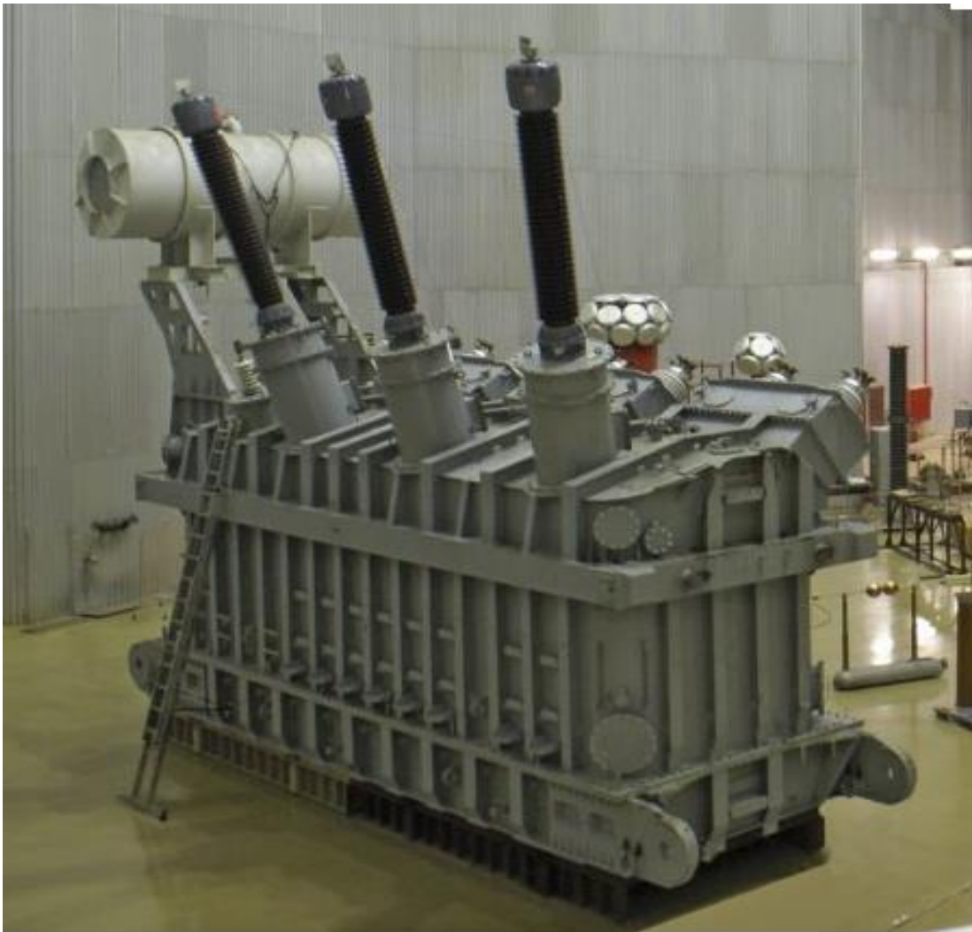
7.1 – rasm. TS-630000/330 tipli kuch transformatori zavodining tajriba zalida
