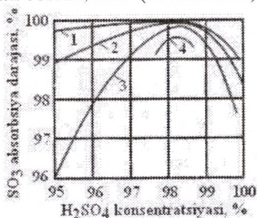
4.14-rasm. Monogidratli absorberda turli haroratda sulfat anhidridning absorbsiyalanish darajasi:
