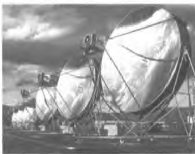
Figure 2.6. Scheme and picture of active solar system concentrators (a) is right-angled, b) is parabolic.
