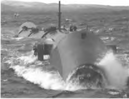
Figure 5.42. The world's largest wave power plant, Agucadoura Wave Farm in Povua de Varzin, Portugal 10 .
