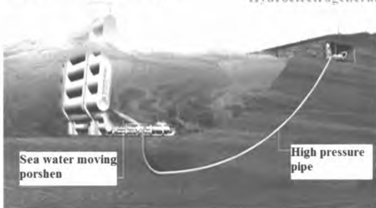
Figure 5.37. The Ustritsa device, which generates electricity using waves.
