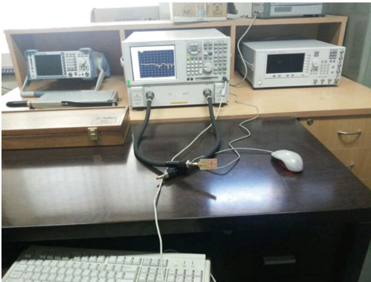
Fig. 10 Antenna connected to network spectrum analyzer
