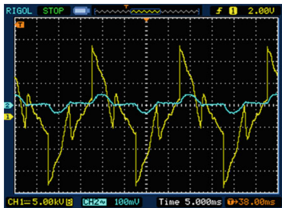
Fig. 8 Output voltage and current waveforms for firing angle = 115^\circ
