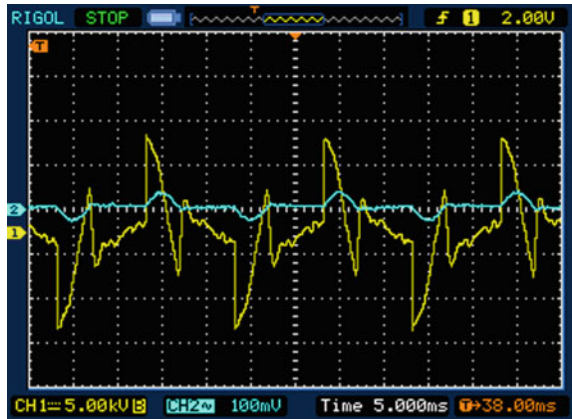
Fig. 10 Output voltage and current waveforms for firing angle = 145°
