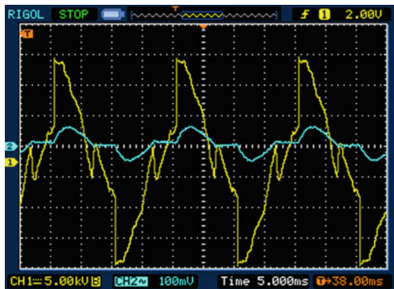
Fig. 6 Output voltage and current waveforms for firing angle = 90°
