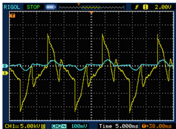
Fig. 9 Output voltage and current waveforms for firing angle = 130^\circ
