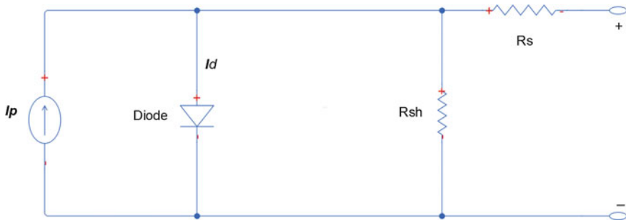
Fig. 1 Equivalent solar cell diagram with a single diode
