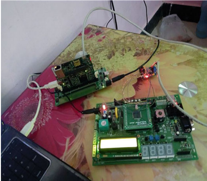
Fig. 3 Interfacing of CAN transmitter and receiver module
