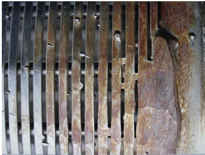
FIGURE 27.8 The stainless steel has rusted where it has been ground and machined.
