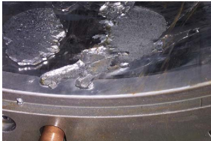
Propeller shaft white metal bearing
