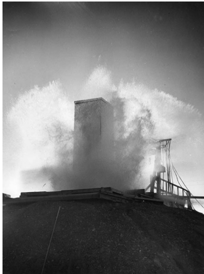
Figure 2.48 Excursion experiment at BORAX-I.
