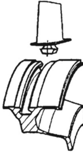
Fig. 13.9 Groove-type method of mounting
