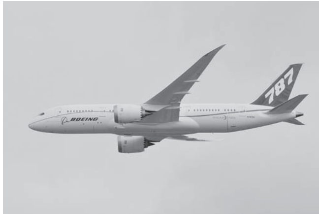
FIGURE 15.9 The Boeing 787 Dreamliner was the first commercial airliner to have composites as the primary material for its airframe construction. (© Jonathan Ayres / Alamy.)
