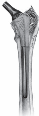
FIGURE 15.7 Prosthetic hip joint. Cutaway artwork of a femur (thigh bone) showing a femoral component of a hip prosthesis. This component is implanted in the femur after the head of the femur has been surgically removed. The upper part of the femoral prosthesis is coated with a thin layer of hydroxyapatite to enhance adhesion to the bone. The other components of the hip joint are a rounded ball to fit into the socket implanted in the patient's pelvis (not shown). This allows the patient to regain mobility, and is usually done to treat severe osteoarthritis or a broken hip. This is an Omnifit prosthesis. (D&L Graphics / Science Source.)
