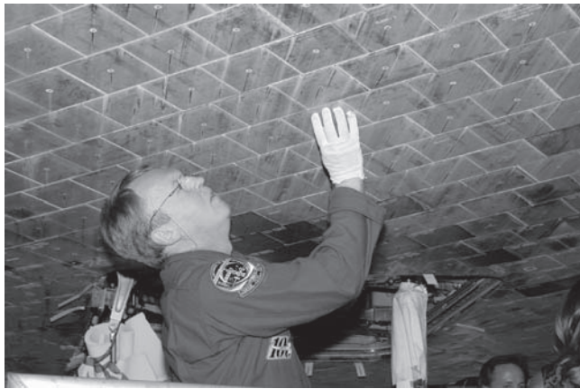
Astronaut Andrew Thomas inspects the ceramic tiles that comprised the thermal protection system (TPS) on the Space Shuttle Orbiter Atlantis, the last shuttle to fly in space. The TPS advanced the state-of-the-art in thermal insulation for the extremely demanding conditions of reentry for the Space Shuttles. (Courtesy of the National Aeronautics and Space Administration [NASA].)
