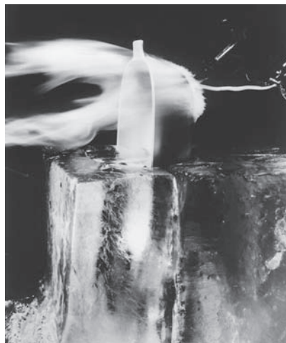
FIGURE 11.2 Cookware made of a glass-ceramic provides good mechanical and thermal properties. The casserole dish can withstand the thermal shock of simultaneous high temperature (the torch flame) and low temperature (the block of ice). (Courtesy of Corning Glass Works.)
