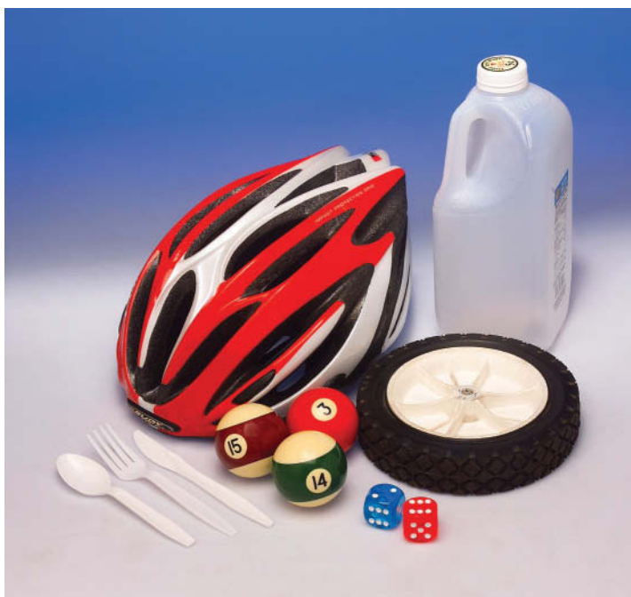
Figure 1.11 Several common objects made of polymeric materials: plastic tableware (spoon, fork, and knife), billiard balls, a bicycle helmet, two dice, a lawn mower wheel (plastic hub and rubber tire), and a plastic milk carton.
