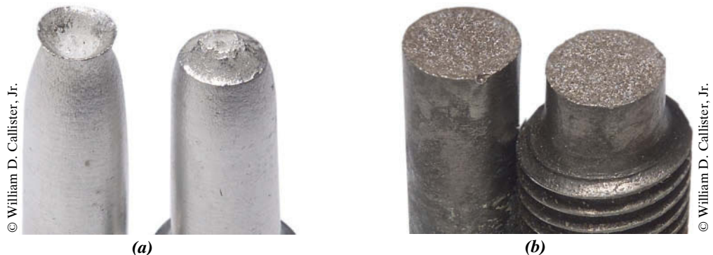
Figure 8.3 (a) Cup-and-cone fracture in aluminum. (b) Brittle fracture in a mild steel.
