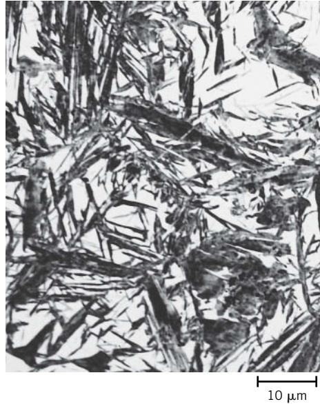
Figure 10.21 Photomicrograph showing the martensitic microstructure. The needle-shape grains are the martensite phase, and the white regions are austenite that failed to transform during the rapid quench. 1220 \times . (Photomicrograph courtesy of United States Steel Corporation.)
