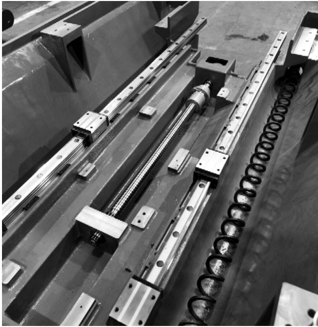
FIGURE 3.49 Typical arrangement of guideways, rolling bearing packs, and ball screw system in a machine bed. (Courtesy of Cincinnati Milacron, Cincinnati, OH.)
