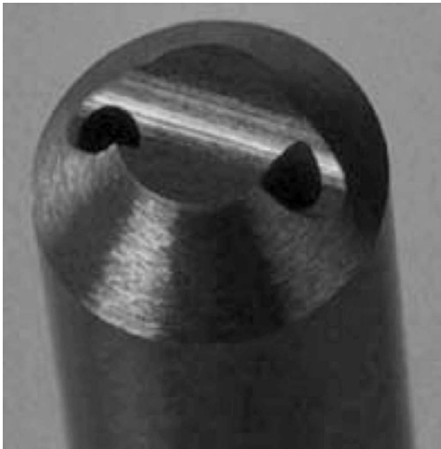
FIGURE 15.10 90° cone MQL shank interface with a wide lubricant slot aligned with the coolant holes. (After Hänle, P., and Schwenck, M., Optimisation of Cutting Tools Using CA-technologies, Proceedings of the Eight CIRP International Workshop on Modeling of Machining Operations , Chemnitz, Germany, 2005, pp. 463–468.)
