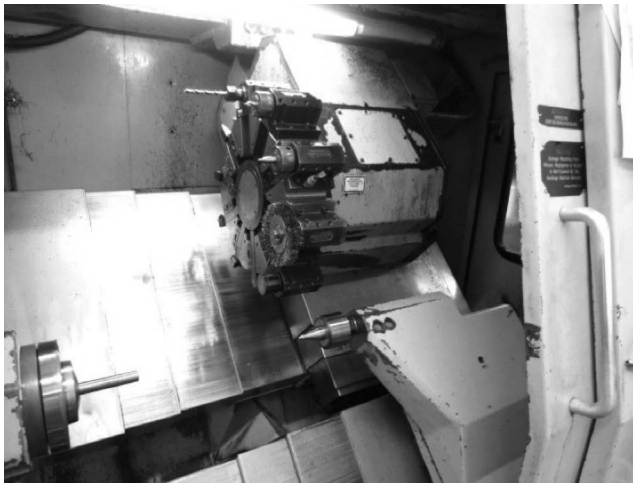
FIGURE 3.7 Interior view of slant bed CNC lathe showing turret, headstock, and tailstock.
