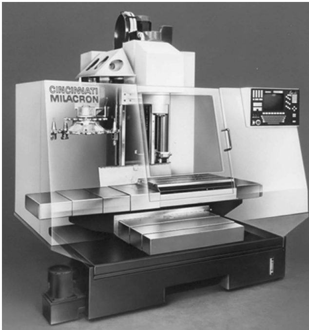
FIGURE 3.10 Solid base, fixed column vertical spindle three-axis machining center. (Courtesy of Cincinnati Milacron, Cincinnati, OH.)
