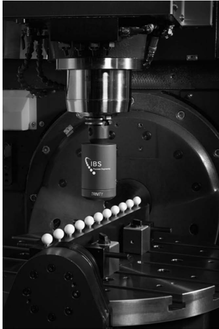
FIGURE 16.28 Illustration of a 2D artifact with precision spheres on a rotary table of five-axis machine tool. (Courtesy of IBS Precision Engineering, Eindhoven, the Netherlands.)
