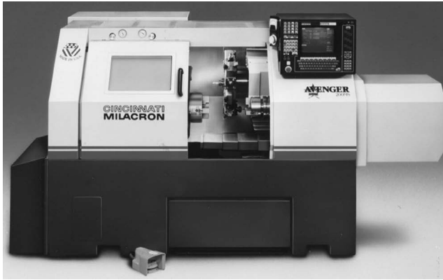
FIGURE 3.6 A CNC turning center with a main spindle and a subspindle for second-side capability, a rotating tooling turret, and a contouring C-axis. (Courtesy of Cincinatti Milacron, Cincinatti, OH.)
