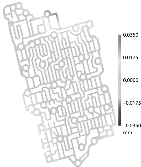
FIGURE 10.24 Illustration of the of the channel surface flatness using the 3D holographic laser method.
