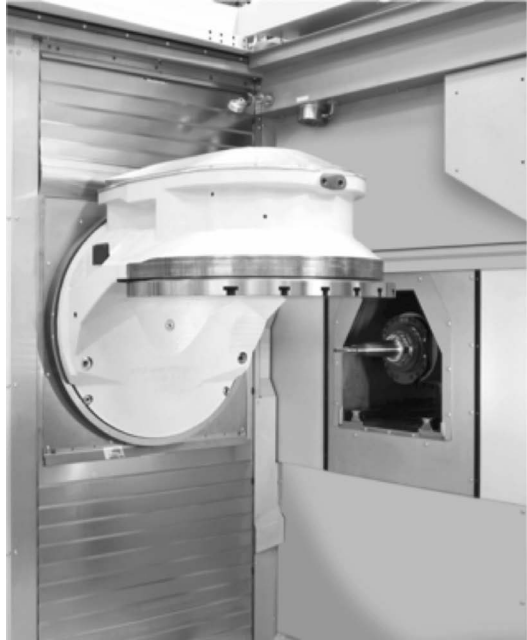
FIGURE 3.15 Horizontal spindle four-axis machining center with A-axis table that can be inverted for MQL machining. (From GROB, Mindelheim, Germany.)
