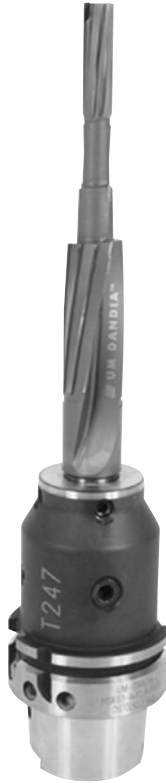
FIGURE 5.69 Steerable toolholder for transmission spool bore reamers and other rotating tools with critical runout requirements. Tightening the two rows of bolts in sequence while measuring runout with an indicator can be used to set up such tools with less than 5\ \mu\text{m} TIR runout. (Courtesy of Kyocera Unimerco, Saline, MI.)
