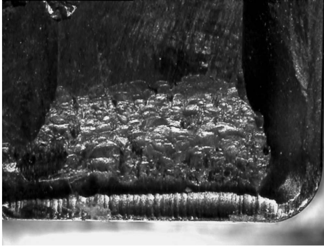
FIGURE 9.12 Chip hammering and cratering on a coated carbide insert used to machine a nickel alloy.
