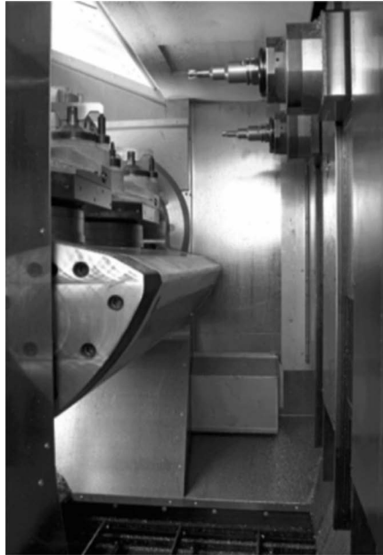
FIGURE 15.8 Interior of a twin spindle MQL machining center, showing horizontal spindle A-axis architecture, steep, unobstructed stainless steel walls, and an open bed over a chip conveyory. (From GROB, Grob Werke, Mindelheim, Germany.)
