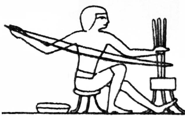
FIGURE 1.2 An early multi-spindle drilling operation in the manufacture of stone beads in ancient Egypt: simultaneous bow-drilling of three beads using a long bow to drive three drills. (Detail of a painting from the tomb of Vizier Rekh-Mi-Re, Thebes, 18th Dynasty, c. 1430 BCE.)
