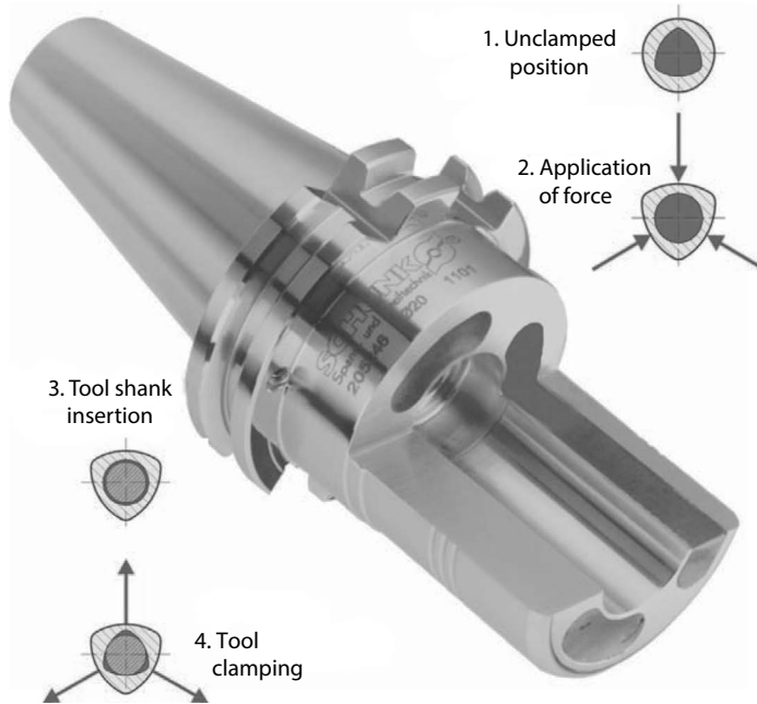
FIGURE 5.67 Precision polygonal mechanical actuated Tribos toolholder chuck. (Courtesy of Schunk Inc., Lauffen/Neckar, Germany.)
