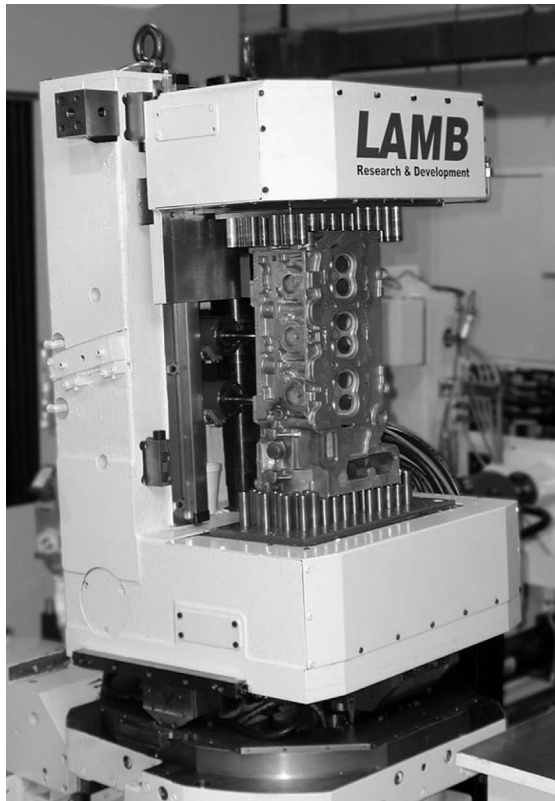
FIGURE 5.94 Bed of Nails fixture shown holding an engine head. (From Lamb Technicon, Warren, MI.)
