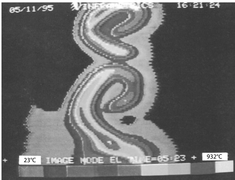
FIGURE 7.9 Full-field infrared thermal image of chip formation when machining 1045 steel at 170 m/min. (Courtesy of I. S. Jawahir, University of Kentucky, Lexington, KY.)
