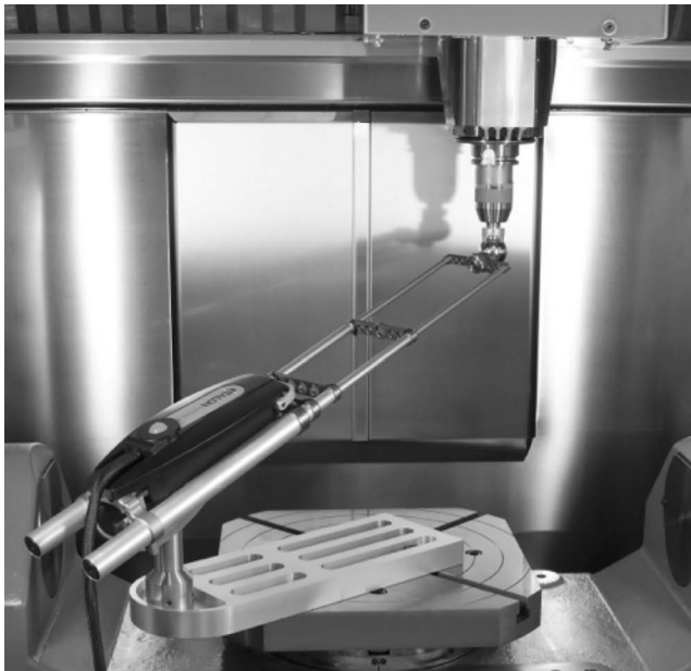
FIGURE 16.15 Illustration of the laser ball bar test on a rotary table of five-axis machine tool. (Courtesy of Etalon AG, Braunschweig, Germany.)
