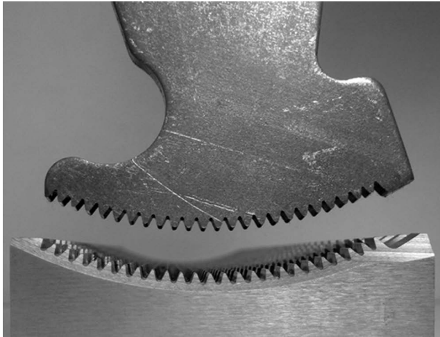
FIGURE 17.8 Surface broach (bottom) used to cut a segment of teeth on a part (top). (From Wolverine Broach Co., Inc., Harrison Charter Township, MI.)
