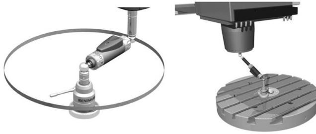
FIGURE 16.13 Illustration of ball bar test in a machine tool. (Courtesy of Renishaw, Hoffman Estates, IL.)
