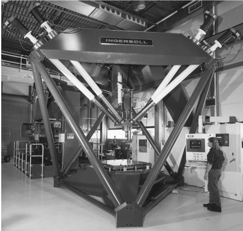
FIGURE 3.36 The structural configuration of the octahedral hexapod machining system (a 6DOF PKM). (Courtesy of Ingersoll Milling Machine Company, Rockford, IL.)
