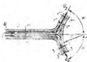
11.1-rasm. Oqimchani to'siqqa urilishi
