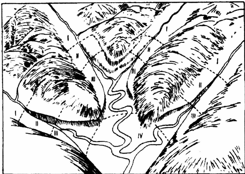
48-rasm. Soyilar sochilmalarining zonalarga ajratilishi (Bilibin, 1955 bo'yicha): I va IV zonalar – vodiy sochilmalari; II zona – terrasalar va o'zan sochilmalari; III zona – o'zan sochilmalarining vodiy sochilmalariga aylanishi va terrasa sochilmalarining yemirilishi.
