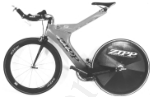
Figure 14.6 High-performance Zipp bicycle with monocoque frame (courtesy of Julian Ormandy, School of Metallurgy and Materials, University of Birmingham, UK).
