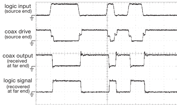
Figure 12.116. Waveforms from a 74AUC1G04 inverter operating at 1.8 V and directly driving a 30 cm length of coax, with the same pulse pattern as earlier, but at a 10 ns clock rate. The four traces (top to bottom) correspond to points A, C, D, and E in Figure 12.114, but with no resistor. The approximate half-step at the coax input confirms a drive impedance close to 50 \Omega . Horizontal: 20 ns/div; vertical: 2 V/div.
