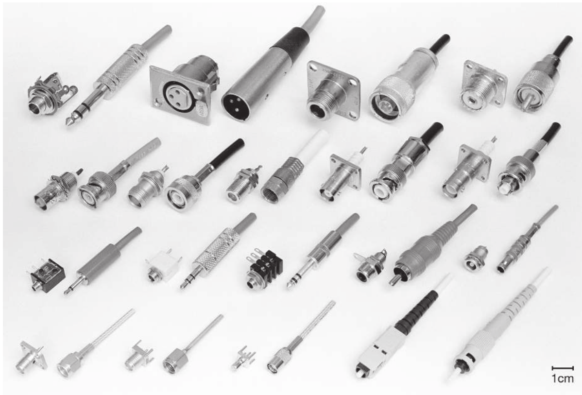
Figure 1.125. RF and shielded connectors. The panel-mounting receptacle is shown to the left of each cable-mounted plug. Top row, left to right: stereo phone jack, audio “XLR” type; N and UHF (RF connectors). Second row down: BNC, TNC, type F; MHV and SHV (high voltage). Third row down: 2.5 mm (3/32”) audio, 3.5 mm stereo, improved 3.5 mm stereo, phono (“RCA type”), LEMO coaxial. Bottom row: SMA (panel jack, flexible coax plug), SMA (board-mount jack, rigid coax plug), SMB; SC and ST (optical fiber).
