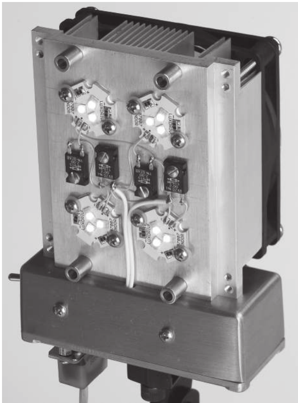
Figure 12.64. Computer CPU heatsink hijacked to make cool desk lamp. We cranked down the current so you can see the four sets of LED triodes, along with the surface-mount ballasting resistors. At full brightness (1000 lumens) you can't look at this thing! The switching driver circuitry of Figure 12.63 lives in the box at bottom.
