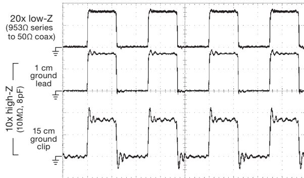
Figure 12.30. Logic waveform at 10 MHz from a 74AC14 inverter running at 3.3 V, as seen on a Tektronix TDS3044B ’scope when probed three different ways. Vertical: 2 V/div; horizontal: 40 ns/div.
