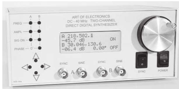
Figure 15.6. Dual DDS frequency synthesizer of Figure 15.5, with panel controls (eleven buttons and one rotary encoder dial) and readout. (Designed, built, coded, and documented with excellence by Jonathan Wolff; see www.artofelectronics.com/synthesizer )
