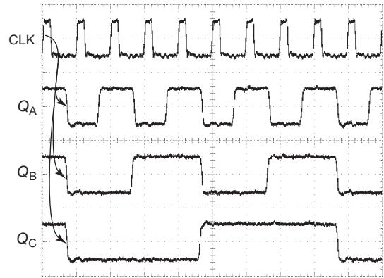
Figure 10.71. In contrast to a ripple counter (Figure 10.62), a synchronous counter (or, indeed, any synchronous system) has all flip-flops clocked from a common source. Here a 74HC161 4-bit synchronous counter (rising-edge triggered) displays a CLK-to- Q delay of about 14 ns, constant for all Q 's, thus producing coincident changes. (Same conditions as Figure 10.63)
