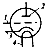
1.2. 1-rasm. Trioidning shartli belgilanishi:
