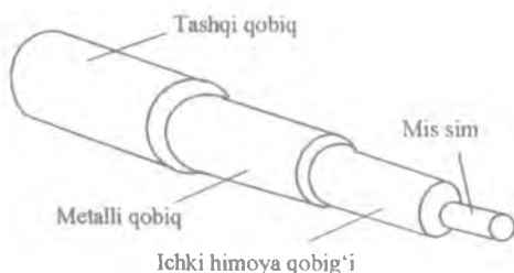
6.2-rasm. Koaksial kabel tuzilishi.
