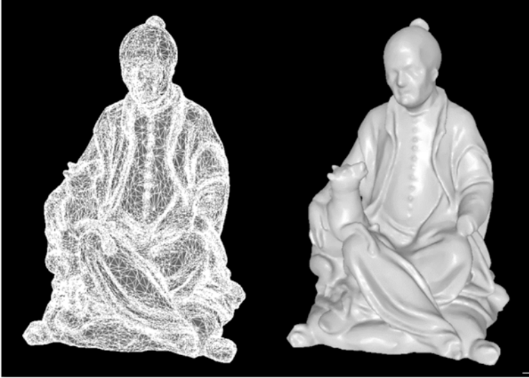
Fig. 3.16 Wireframe versus surface model [4]
