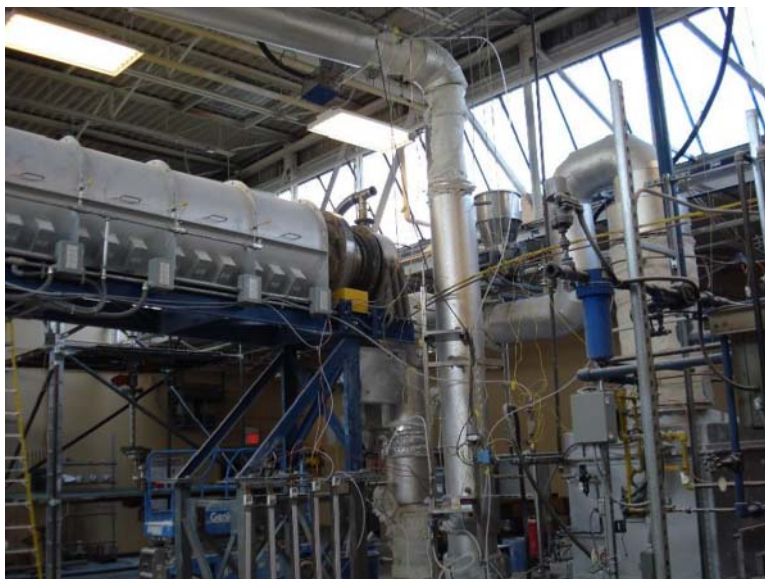
Figure 13.5 Photo of 120 kW –calcination reaction (CCR) process facility for CO 2 and SO 2 capture at Ohio State University initiated in 2005 with coal-fired stoker, rotary calciner, and entrained bed carbonator shown and with the same facility used also for Carbonation–Calcium–Hydration Cyclic Process operation. Source: With permission from Professor L-S. Fan at Ohio State University.
